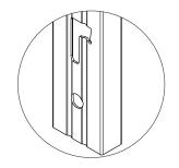
Step 8 - Mark wall connector hole location onto wall. Each hole requires mounting hardware. Set wall connector aside.
