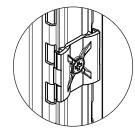
Step 2 - Snap end trim extrusion over clips.
